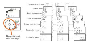
Navigating the menu structure (e.g. special parameters, monitoring signals)
