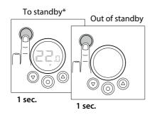
\*The heat is not being regulated. The clock is running and any settings are saved in the memory.
