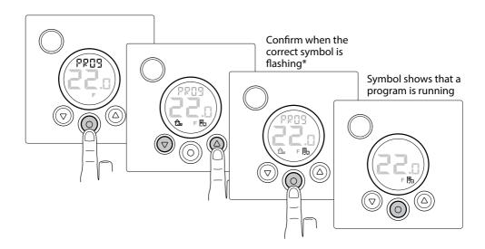
\*Stop program: Confirm when no symbol is flashing.
