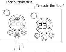
\*If the thermostat is set to *Floor thermostat*. Otherwise the room temperature (R) is displayed.
