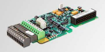
Use this feedback option board to connect 2 HTL type pulse/incremental encoders to an NXP product.
