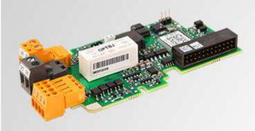
This option board provides the VACON® 100 product with the Safe Torque Off (STO) safety function. The option board also features an ATEX thermistor input for protection against motor overtemperature, where the motor is located in an ATEX environment. One relay output is also available for indicating STO function.
