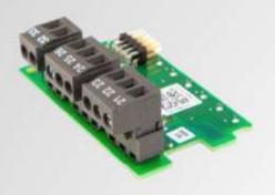
This I/O option board provides relay outputs to the VACON® 100 HVAC products using old control cards.
