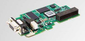
This option board provides PROFIBUS DP-V1 interface to VACON® 100 and VACON® 20 product families. The option board is identical to OPT-E3 apart from the fieldbus connector.
