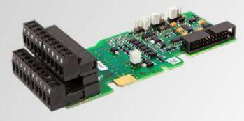
This I/O option board for the NXS and NXP products provides a variety of input and output signals for controlling the drive. It is equivalent to OPT-A1 except that in OPT-A9 the connectors have a cross-section of 2.5 mm<sup>2</sup>.
