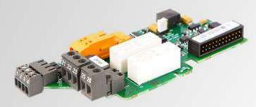
This option board provides the NXP product with the Safe Torque Off (STO) safety function. The option board also features an ATEX thermistor input for protection against motor overtemperature, where the motor is located in an ATEX environment. 2 relay outputs are also available in the option board.
