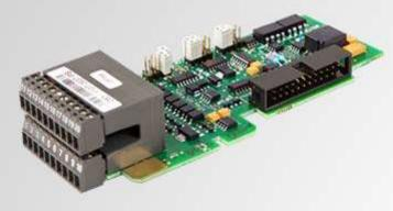
This I/O option board for the NXS and NXP products provides a variety of input and output signals for controlling the drive. It is equivalent to OPT-A1 except that analog inputs and outputs are galvanically isolated in OPT-A8.
