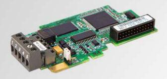
This option board provides a DeviceNet<sup>TM</sup> interface to VACON®  $NX_{-}$  products.
