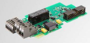
This I/O option board for the NXL product provides a variety of input and output signals for controlling the drive.
