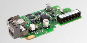
This adapter option board enables connection of VACON® NXP drives via fiber-optic cables. Use the link for drive-to-drive communication or for parallelling of drives to achieve higher power. The board also includes a CAN interface for monitoring of multiple drives, for customized CAN communication or for I/O expansion.
