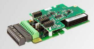
Use this option board to enable speed feedback to an NXP drive from an EnDat 2 encoder. Use the EnDat interface to read the absolute position of the shaft. The option board outputs a simulated pulse encoder signal according to RS422 specification.
