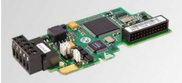
This option board provides a PROFIBUS DP-V0 interface to NX\_ products. The option board is identical to OPT-C5 apart from the fieldbus connector.
