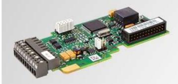
Use this option board to enable speed feedback to an NXP product from an EnDat 2.1 encoder. Use the EnDat or SSI interface to read the absolute position of the shaft.
