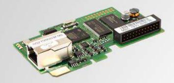
This option board provides a PROFINET interface to VACON® NX\_ products.
