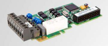
This I/O option board provides five high-voltage digital inputs and one relay output to VACON® AC drives. The option board can be used in VACON® NX\_ products and also in VACON® 100 and VACON® 20 product series.
