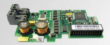
This option board provides VACON® AC drives with an AS-i bus interface.
