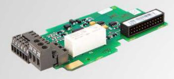
This I/O option board for the NXL product provides a variety of input and output signals for controlling the drive.
