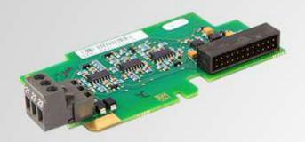
This adapter option board provides VACON® NXP drives with an interface for measuring mains/line voltage. The board includes a transformer to reduce the line voltage to a measurable amplitude. The board is used in applications such as AFE, renewable energy or microgrid.
