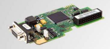
This option board provides a multiprotocol RS-485 interface to VACON® NX\_ products. The option board is identical to OPT-C2 apart from the fieldbus connector.
