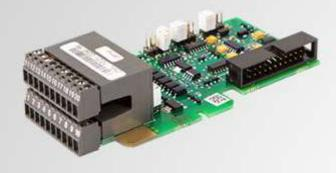
This I/O option board for the NXS and NXP products provides a variety of input and output signals for controlling the drive:
