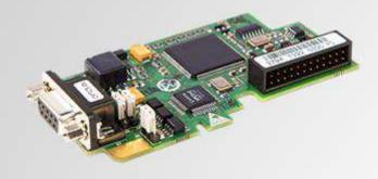
This option board provides a PROFIBUS DP-V0 interface to VACON® NX\_ products. The option board is identical to OPT-C3 apart from the fieldbus connector.
