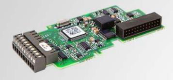
This I/O option board provides three temperature measurement channels to VACON® AC drives. The option board can be used in NXS, NXP and in VACON® 100 products.
