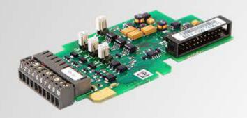
Use this feedback option board to connect NXP products to HTL type pulse/incremental encoders.
