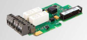
This I/O option board for the NXS and NXP products provides 2 relay output signals and a thermistor input for overtemperature protection:
