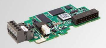
This option board provides a PROFIBUS DP-V1 interface to VACON® 100 and VACON® 20 product families. The option board is identical to OPT-E5 apart from the fieldbus connector.
