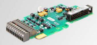
Use this feedback option board to connect HTL-type pulse/incremental encoders to NXP products.
