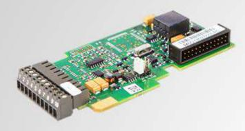
Use this feedback option board to connect sine/cosine type incremental encoders to an NXP product.
