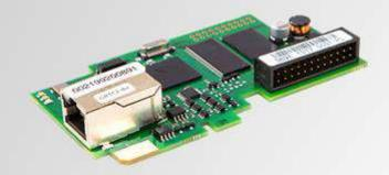
This option board provides Modbus TCP interface to VACON® NX\_ products.
