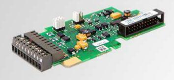
Use this feedback option board to connect NXP products to TTL and TTL(R) type pulse/incremental encoders conforming to the RS422 specification.
