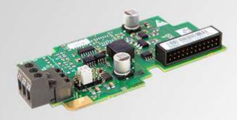
This adapter option board supplies a CAN interface to the IEC 61131 application of VACON® NXP drives. Use the CAN interface for monitoring of multiple drives, for customized CAN communication or for I/O expansion.
