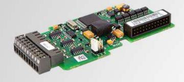
This I/O option board provides three temperature measurement channels to VACON® NXS and NXP drives.
