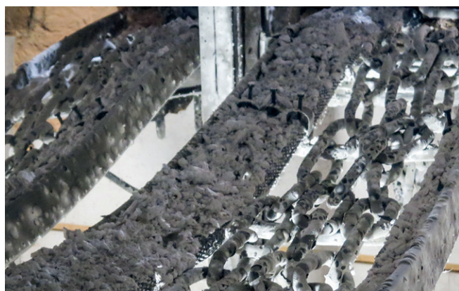
KS80-400 cable ladder after a 60-min fire test.
