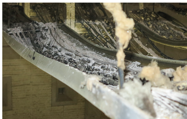
KRA cable ladder after a 90-min fire test.
