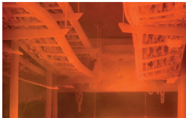
60 min after the start of the fire test: the temperature in the furnace is approx. 950 °C. The cable ladder on the bottom left of the image has been fastened with an interval of 2 m, and above that, the fastening interval is 1.2 m (a sample of deflection).
