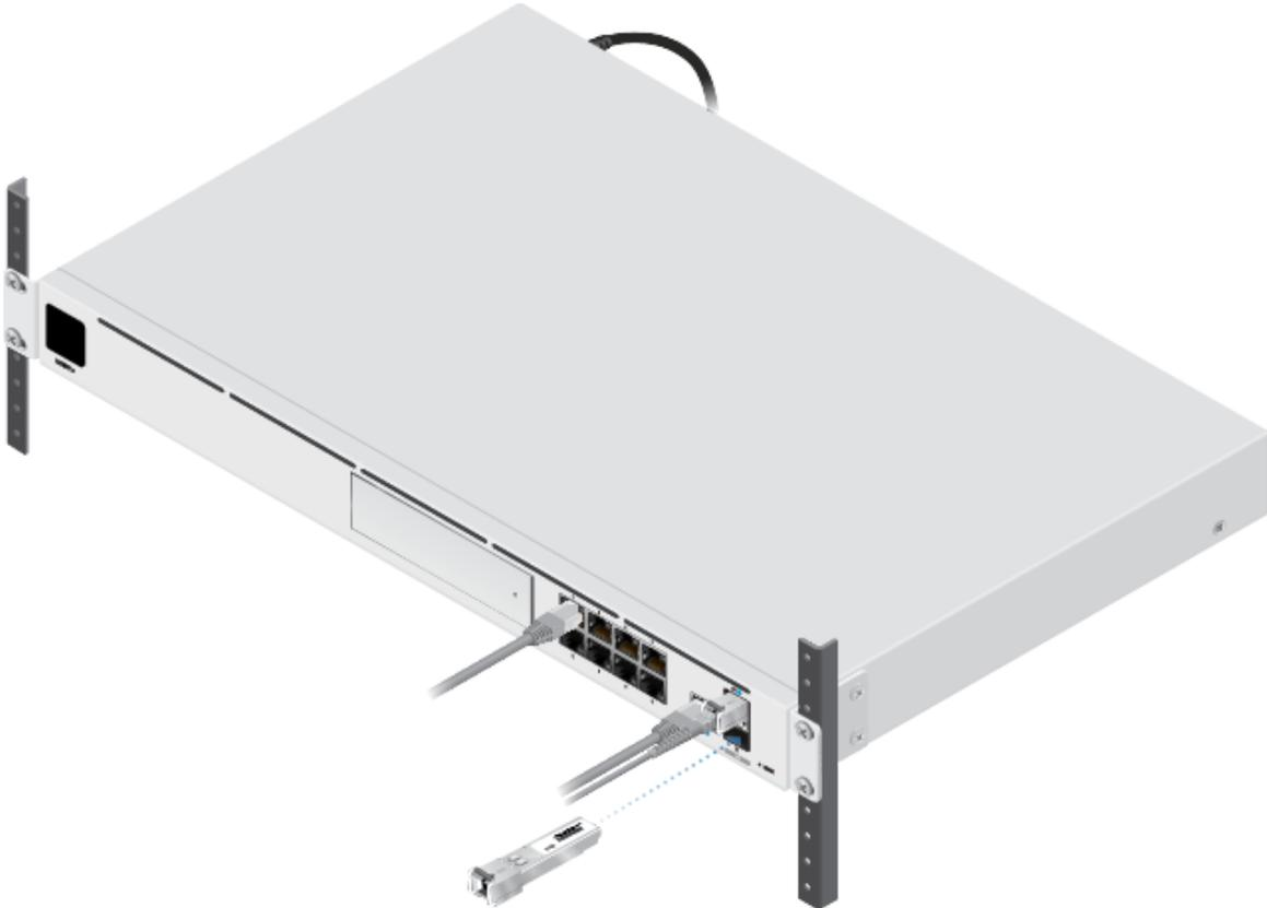
4. Connect the other end of your fiber optic cable to the SFP Fiber Module.
