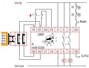
Figure 45 - With Two Devices with Mechanical Contacts and Monitored Manual Reset
