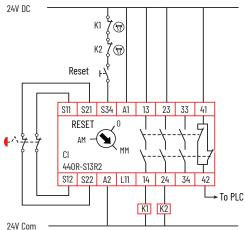
The following image shows a CI safety relay monitoring a safety light curtain with two OSSD outputs. The CI safety relay is set to automatic/manual reset (AM). The auxiliary signal (terminals 41/41) informs the PLC that the safety system is off or on. The CI safety relay outputs connect to AC voltage loads. When the CI safety relay is on, the PLC can then turn on the K1 and K2 contactors.
