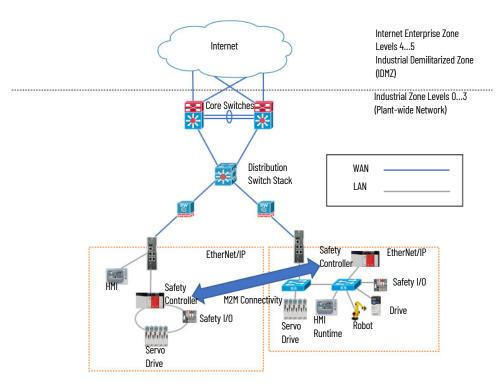
The following architecture is highlighting the use of the Stratix 4300 for remote access purposes. An IES is positioned in the cell for any other North/South and East/West traffic. The IES switching infrastructure also provides routing and switching services to all devices including the Stratix 4300. The VLAN required for Internet access or WAN must be extended into the cell/area zone IES to provide this is to verify that the Stratix 4300 has Internet access for remote access.
