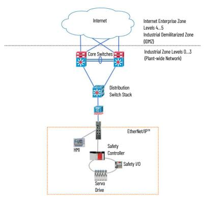
The following architecture is highlighting the use of the Stratix 4300 for remote access purposes and NAT/Routing purposes. The Stratix 4300 provides remote access to each individual cell/area zone. If there is a need for peer-to-peer or machine-to-machine communication, the Stratix 4300 NAT or Routing features can be configured to allow successful communication.
