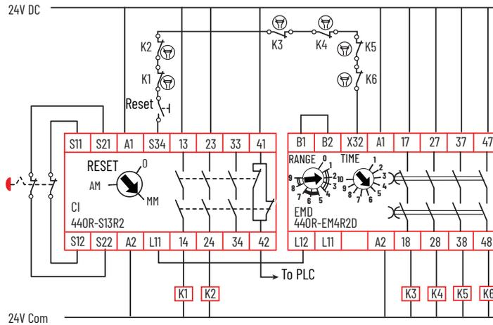
The following image shows the EMD safety relay that is configured for a 2.1 second on-delay. The single wire safety signal from terminals L11 to L12 instructs the EMD safety relay to turn on and off. When the Reset button is pressed, the DIS safety relay outputs turn on immediately. After a 2.1 second delay, the EMD safety relay outputs turn on.
