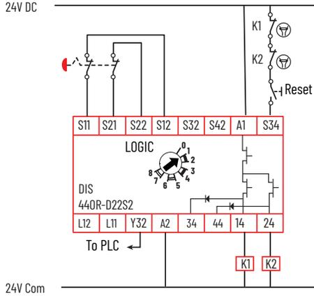
The DIS safety relay monitors two devices with OSSD outputs in the following image. The DIS safety relay logic setting is 6: (IN1 AND IN2) OR L12 with automatic reset. The output terminals 34 and 44 are designed to tolerate higher capacitance loads (but lower resistive load) as compared to terminals 14 and 24.
