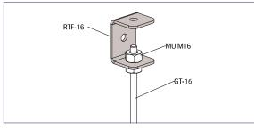
Ceiling bracket RTF-16 is attached to threaded rod GT-10 or GT-16 and nuts MU M10 or MU M16, depending on the orientation of the ceiling bracket.
