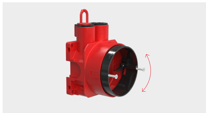
04 An optimal height for the top surface of the box is achieved by using the adjustable installation ring. This allows the device to be installed parallel with the wall's outer surface.
