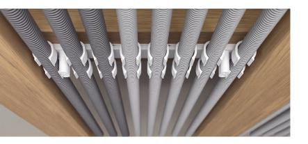
Halogen free fastening list for 16 pcs of flexible or rigid conduits (16/20 mm). List can be cut to needed length and attached on top of the other. Ideal for fastening and organizing conduits.
