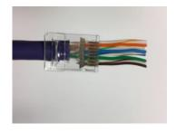
Whilst gripping the wires to ensure they do not get crossed, feed them through the connector so all 8 protrude out of the front of the connector as shown. Push the cable jacket into the back of the connector as shown
