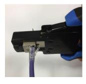
Slide the boot up to locate in the back of the connector and feed the connector into the crimp tool as shown. Ensure the connector is pushed all the way in until it latches into the tool
