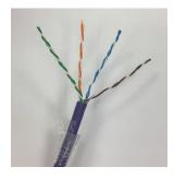
Carefully cut off the wire separator close to the cable jacket (within 2mm). Take care not to cut the wires
