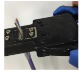
Crimp the connector. The crimp tool will simultaneously crimp the cable, retain the boot, crimp the 8 contacts to the wires and cut the wires flush
