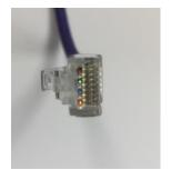
Remove the connector from the crimp tool. The wires are all neatly cut and flush with the front of the connector
