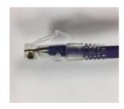
Completed termination showing correct positions of the boot, cable and wires
