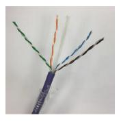
Splay the wires out to reveal the wire separator
