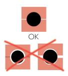
5 The diagram marked OK shows how the cable should look when correctly fitted.
