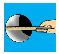
Measure the opening and check that the measurement is within tolerance. The hole tolerance is equal to the outer diameter of the frame -0/+2 mm.
