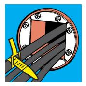
a Position the RGP frame correctly in the opening. Check that the frame is clean and pull through the cables. Position the largest cables at the bottom. Measure the diameter of the cables and choose suitable blocks.
