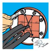
**7** Tighten the nuts diagonally until 12-15 mm of thread is visible.
