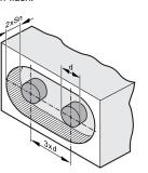
The minimum distance between units may only be disregarded for units with different oscillator frequencies or different sensing principles.
